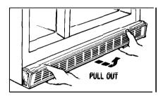
**To adjust rollers,** remove the base grille by grasping it at the bottom and pulling it out.
